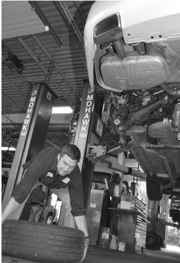
FIGURE 1.1 Worker moves a 125-lb tire manually, resulting in a poor lifting posture. Source: Mohawk Lifts, LLC
