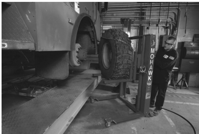
FIGURE 1.2 A tire dolly, does much of the manual work and results in a safer task. Source: Courtesy of Mohawk Lifts, LLC
