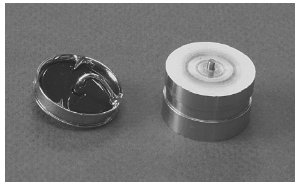
■ Figure 1.2 A mechanical heart valve on the left and the titanium workpiece from which the circular frame of the valve is machined on the right.
