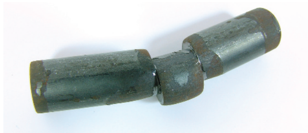
FIGURE 1.4 Double-shear failure in a pin specimen.
