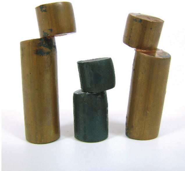
FIGURE 1.3 Single-shear failure in pin specimens.
