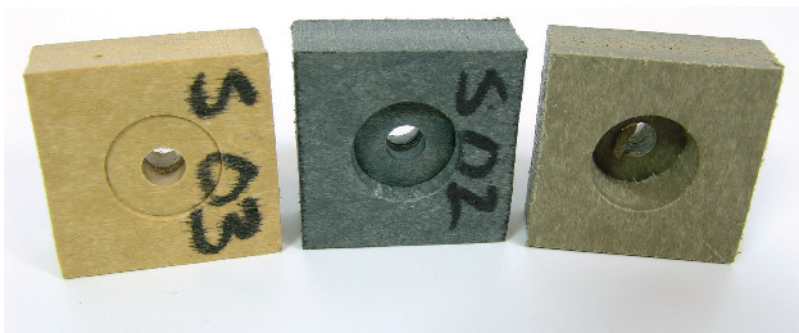
FIGURE 1.5 Punching shear failure in composite wood block specimens.
