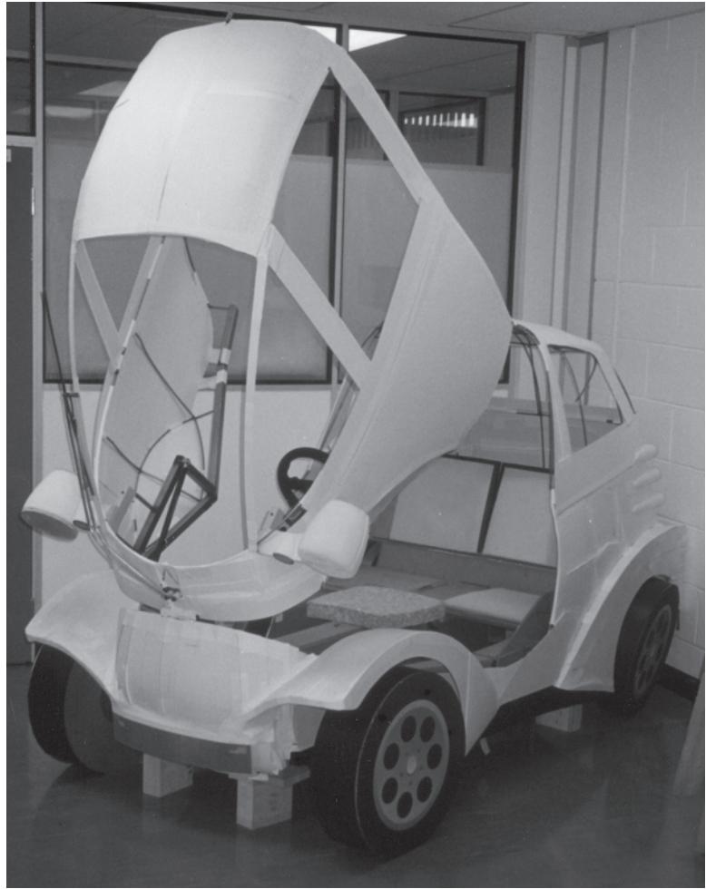
Figure 1.3 A wire and cardboard early-stage mock-up. Source: Gordon Murray; Photo: Nigel Cross.
