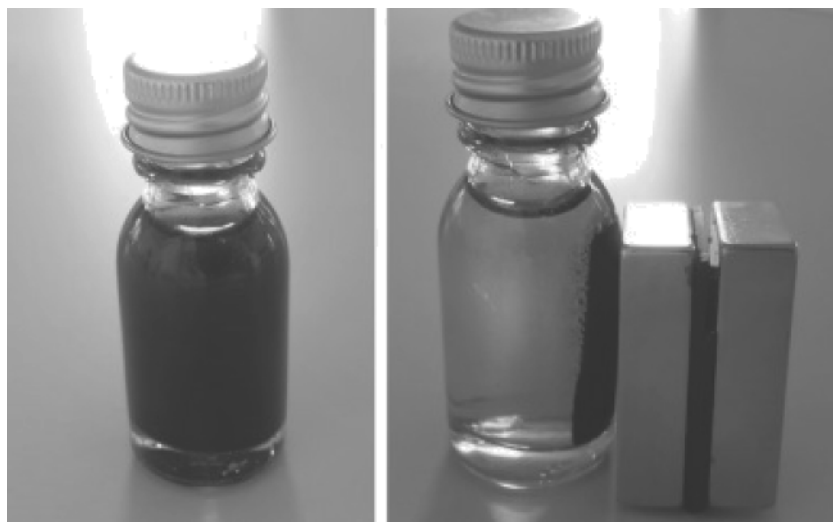
Figure 1.7 Magnetic separation of the magnetic adsorbents during adsorption processes. Reprinted and reproduced with permission from Ref. [94].
