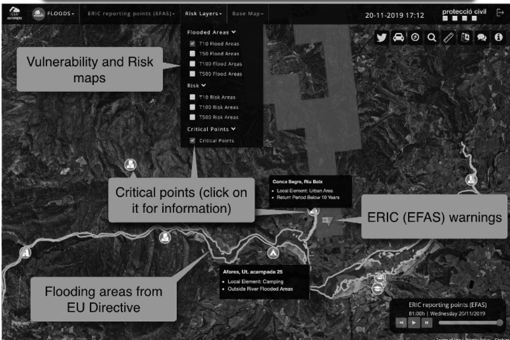
Figure 1.6 Impact forecasting implemented on the A4EU platform, showing critical points that are at risk, by automatic integration of the MHEWS forecasts with high-resolution impact models and the local vulnerability and exposure cartographies. The figure shows how the flash-flood early warning product ERIC (from EFAS) can be used to trigger an automatic warn to the predefined critical points potentially affected using the risk flood maps prepared under the Flood Directive.
