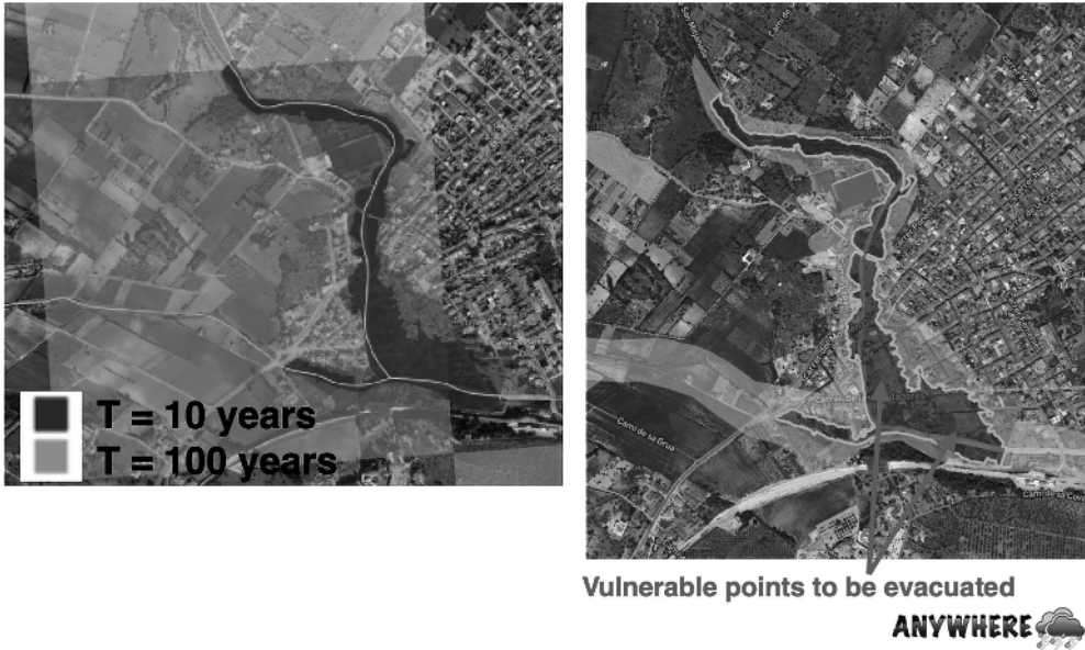
Figure 1.7 (Above) Scheme of the automatic activation of priority actions on the most vulnerable points for the A4EU flash flood impact forecasting. The pre-identified vulnerable points are labelled (Courtesy of HYDS). (Below) Application to the event of 9 October 2018 in Mallorca Island (ES). The orange pixel (1×1km) is the trigger for a flash flood warning over 10-year return period. The Flood Directive risk map allows the system to identify the associated area to be flooded and the vulnerable buildings in which the self-protection protocols should be activated.
