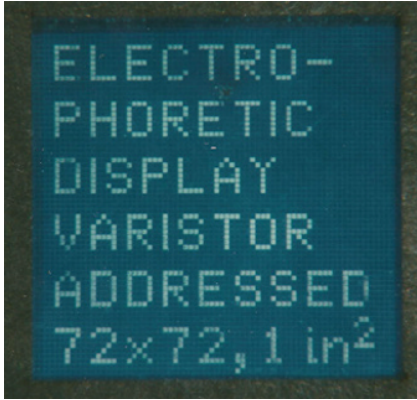
Figure 1.12 Demonstration of the first active-matrix electrophoretic display.
