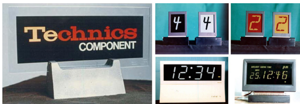
Figure 1.11 First EPD product for point-of-purchase (POP) use, and the experimental numeral display EPD [70] / U.S Patents / Public Domain.
