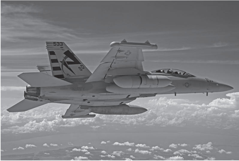
Figure 1.3 The US Navy is employing AESA technology on the Next Generation Jammer mid-band pods for the EA-18G Growler. (US Navy photo by Erik Hildebrandt)
