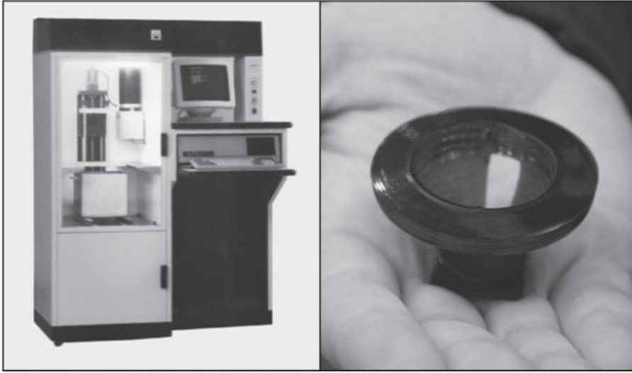
Figure 1.1 First Stereolithography Machine and First 3D Printed Part
