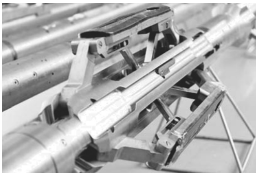
Figure 1.13. New COSL azimuthal triple probe formation tester.
