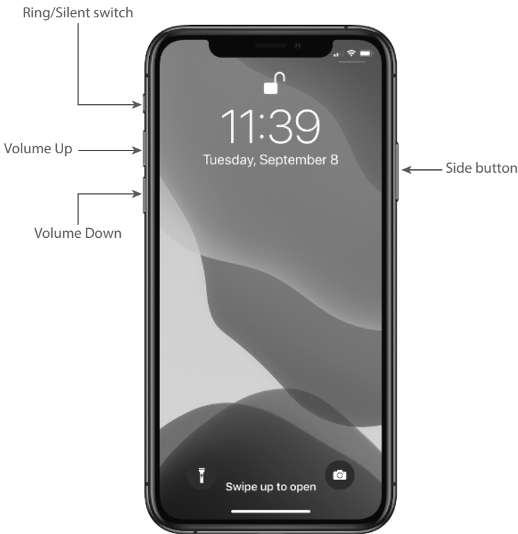
1.1 On all recent iPhone models, the Side button appears on the right side.
