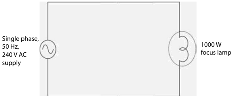
Figure 1.40 Single-phase circuit powering 1000 W focus lamp.
