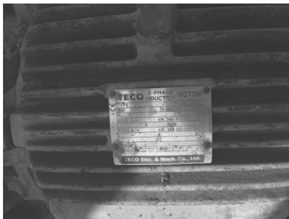
Figure 1.30 Name plate details of three phase induction motor (Courtesy: TECO).
