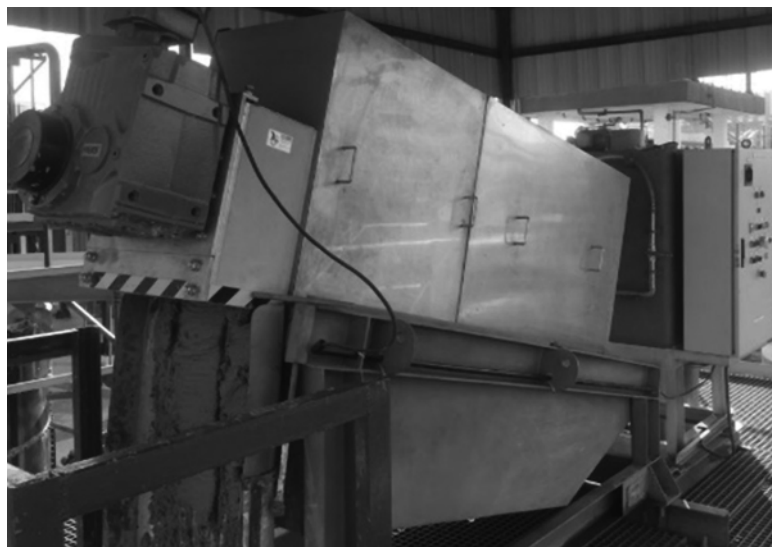
Figure 1.8 Volute press equipment.
