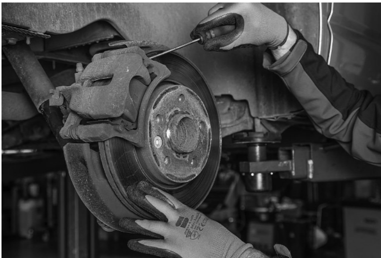
Figure 1.22 Inspection of a brake disc. Source: geraldoswald62/Pixabay.
