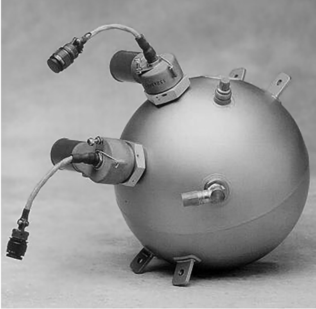
Figure 1.25 Fire extinguisher of aircraft engines. Source: AviationNuggets.
