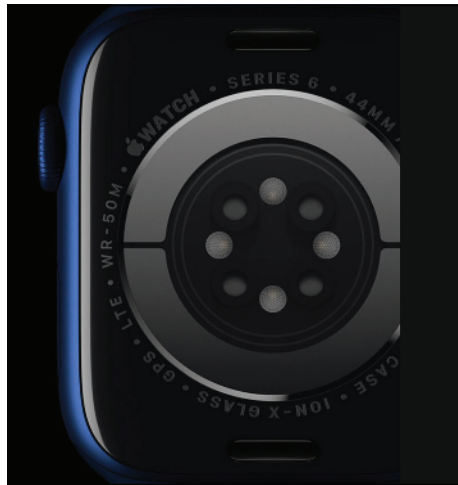
FIGURE 1-11: The sensors on the back of Apple Watch can, among other things, calculate your heart rate and measure your blood-oxygen percentage.
