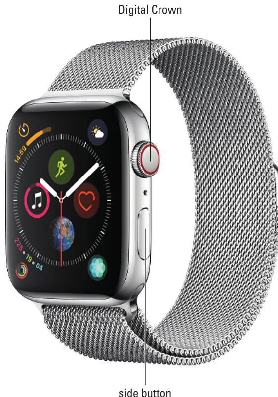
FIGURE 1-10: If worn on the left wrist, the side button is on the right-hand side of the watch case. The Digital Crown button is the ridged dial.
