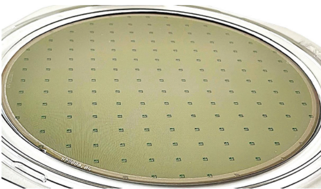
Figure 1.12 A fully processed VCSEL layer structure on 6" (150 mm) GaAs substrate. Source: Wafer photo by Jim A. Tatum, Dallas, Texas, USA. [copyright reserved].
