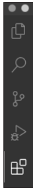
FIGURE 1-3: The Extensions icon is located at the bottom of the Activity Bar.
