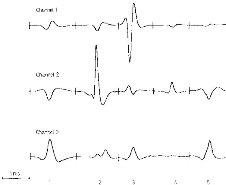
Figure 1.17 SMUAP trains recorded simultaneously from three channels of needle electrodes. Observe the different shapes of the same SMUAPs (aligned vertically across the three channels) projected on to the axes of the three channels. Three different motor units are active over the duration of the signals illustrated. Reproduced with permission from B. Mambrito and C.J. de Luca, Acquisition and decomposition of the EMG signal, in Progress in Clinical Neurophysiology , Volume 10: Computer-aided Electromyography , Editor: J.E. Desmedt, pp 52–72, 1983. ©S. Karger AG, Basel, Switzerland.
