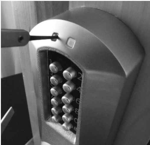
Figure 1-6: The Kaba 5800 electronic push-button lock could be defeated in six ways. I demonstrated these attacks at DefCon. One serious design failure was demonstrated by the insertion of a pin, wire, or pick tip through an LED mount to ground a contact on the PC board. This sent a remote opening signal to an electric strike at the door.
