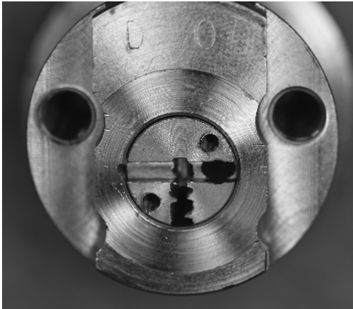
Figure 1-8: Open keyways, as shown in this deadbolt lock, can provide access to wires, shims, and other tools to manipulate a tailpiece.
