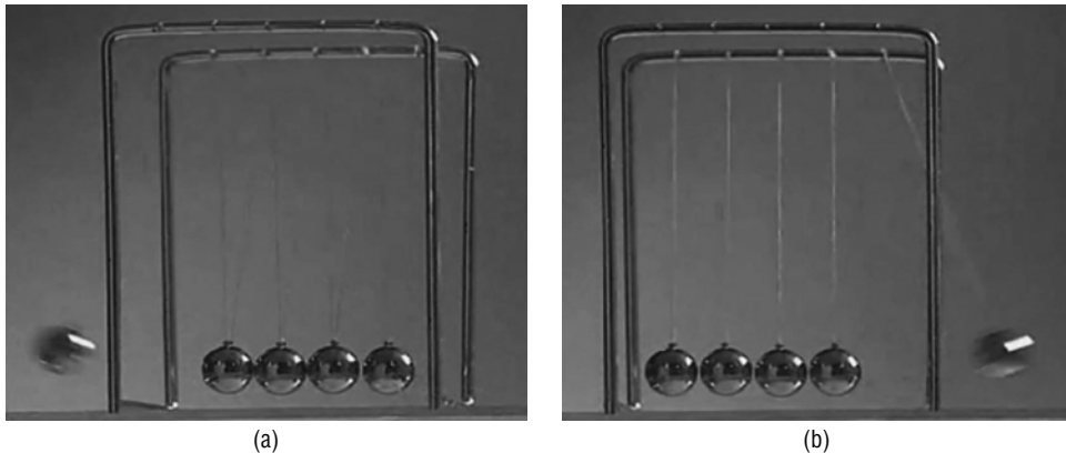
Figure 1-12a, 12b: The classic way to describe Newton's Third Law of Motion is with steel free-swinging balls. (a) The four balls are struck, and (b) the ball on the right is moved because of the energy transmitted as an equal reaction. This is the same theory of lock bumping with pin tumblers. When energy is applied to the base of pins by the key, the reaction causes them to move vertically across the shear line.
