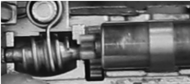
Figure 1-3: A worm gear is controlled by a small motor in electronic locks. The gear is turned when the motor is activated, which causes the gear to advance or retract a locking component.
