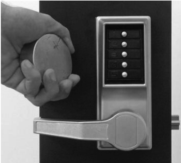
Figure 1-11: The Kaba Simplex 1000 mechanical lock was defeated by a rare earth magnet in seconds because a critical component that controlled unlocking was made of a ferrous material. Moving the round magnet near the lock was all that was required.
