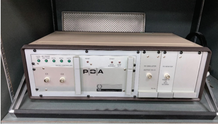
Figure 1.4 Photograph of the first commercial digital PD instrument that measured PD in the 30–300 MHz range. The PDA-H, introduced in 1986, measured the PD from a pair of permanently-installed 80 pF couplers in each phase of an operating hydro generator. The instrument was controlled by an early PC, which also served as the display device. Source: Mladen Sasic, Iris Power L.P.
