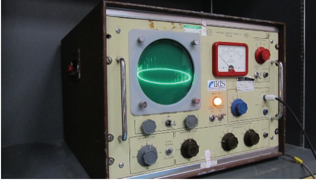
Figure 1.2 Recent photograph of a still-working ERA Model 3S, manufactured by Robinson Instruments, probably in the late 1970s. The instrument was first owned and used by the former British utility the CEGB, before being acquired by Iris Power in the 1990s for its museum. The oscilloscope screen shows the typical elliptical trace of a 60 Hz sinewave with PD from a twisted pair of insulated wires superimposed on it. Source: Mladen Sasic, Iris Power L.P.
