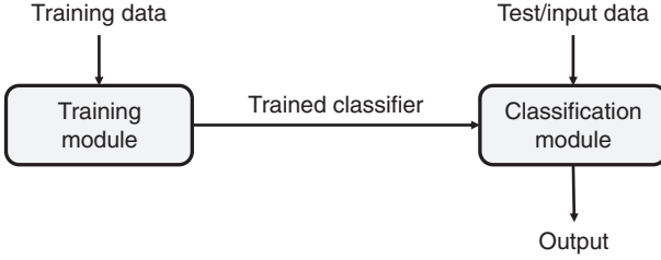
Figure 1.1 A data-driven ML architecture.
