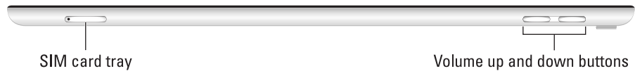
FIGURE 1-3: The right side of the iPad features volume buttons, and some feature a SIM tray, too.
