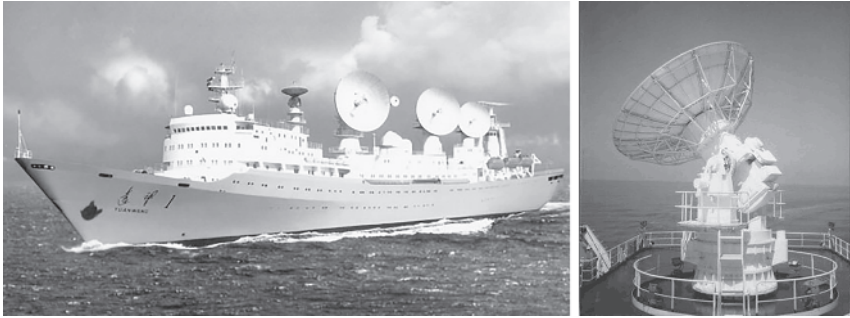
Figure 1.5 The Yuan Wang ocean survey ship and antenna. Source: (a) baike.com.
