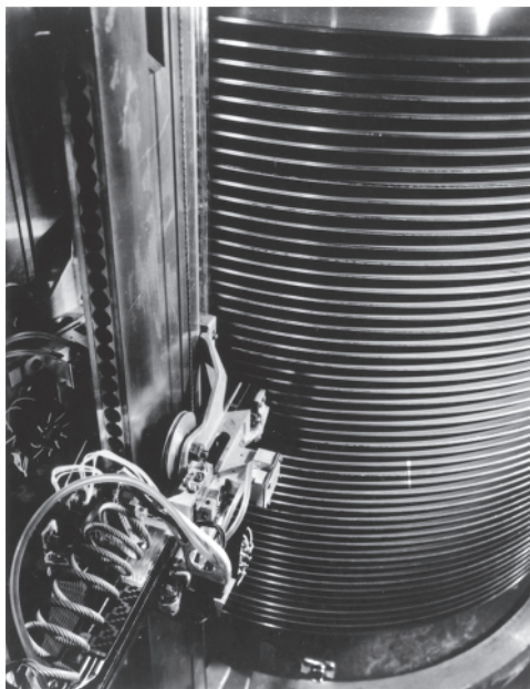
FIGURE 1.8 IBM RAMAC disk storage device, circa 1956
