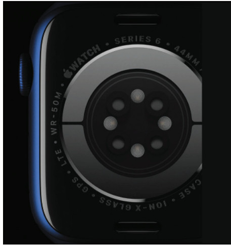
FIGURE 1-12: The sensors on the back of Apple Watch can, among other things, calculate your heart rate and measure your blood-oxygen percentage.
