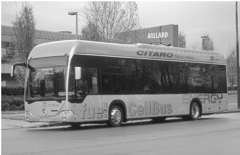
Figure 1.17 Citaro fuel-cell-powered bus, one of a fleet that entered service in 2003 (Photograph reproduced by kind permission of Ballard Power Systems)
