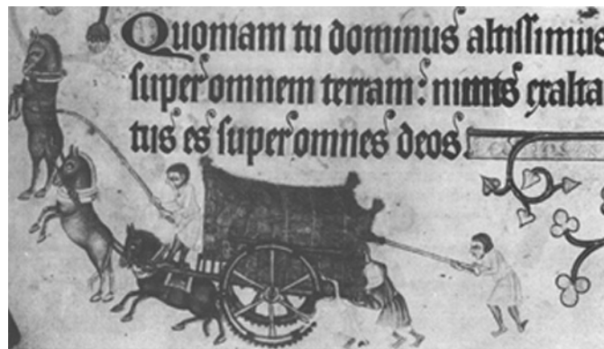
Figure 1.1.1 Drawing of two-wheeled harvest cart with studded wheels. Luttrell Psalter (folio 173v), circa 1338 AD.
