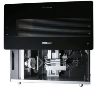
Milling Blanks with Five Axis Milling Machine
