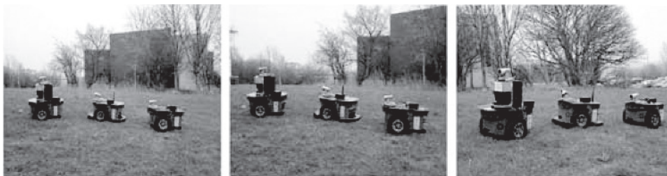
Figure 1.3 Autonomous UGVs (laboratory-scale mobile robot Pioneer3DX) in a convoy formation outside Infolab21, Lancaster University campus
