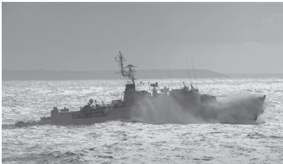
**Figure 1.3 Hydrodynamic impact.** Among many phenomena involving fluid and structure motions in extreme conditions, *slamming* is one of the most spectacular examples of fluid–structure interaction. When sailing at high speed and/or in rough sea condition, the impact of a ship on water induces high loads on the structure: slamming is, among other cases, of primary concern when designing ships. *Source:* © A.Monot/Marine Nationale
