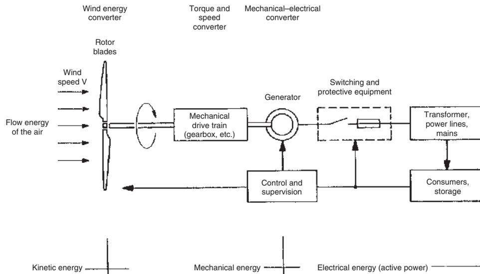
**Figure 1.37** Functional chain and conversion stages of a wind energy converter
