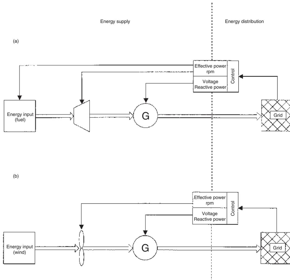
**Figure 1.1** Energy delivery and control in electrical supply systems: (a) diesel generators, etc., and (b) wind turbines
