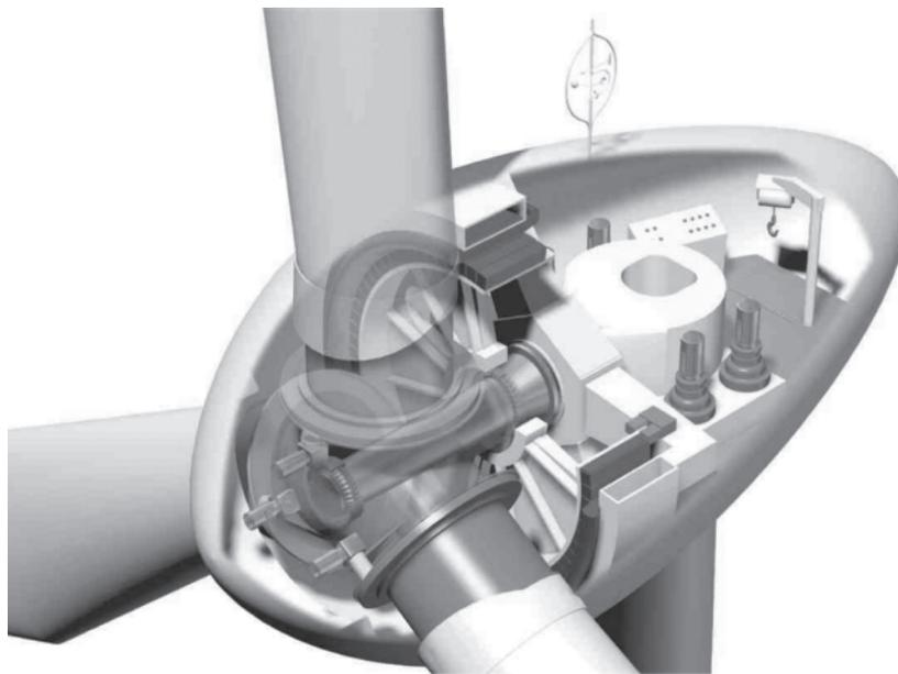
**Figure 1.3** Schematic structure of a gearless wind turbine (Enercon E66, 70 m rotor diameter, 1.8/2 MW nominal output). Reproduced by permission of Enercon
