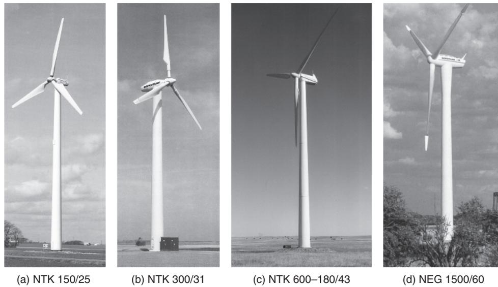
**Figure 1.22** Size progression of stall-regulated turbines of the same design (fixed-speed, fixed-pitch machines) from NEG Micon / Nordtank. Reproduced by kind permission of NEG Micon
