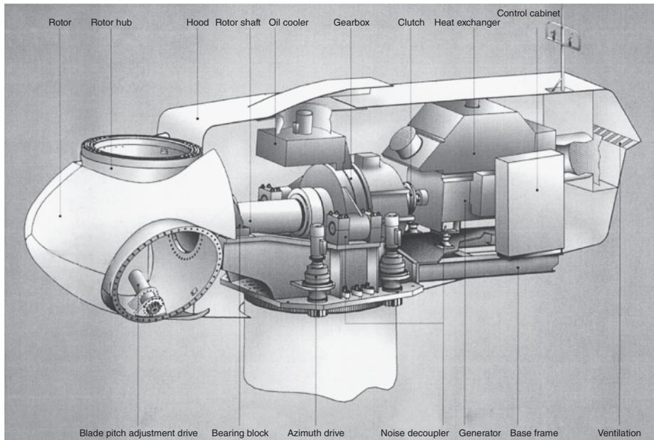
**Figure 1.2** Nacelle of a wind turbine with a gearbox and high-speed 1.5 MW generator (TW 1.5 GE/Tacke). Reproduced by permission of Tacke Windenergie
