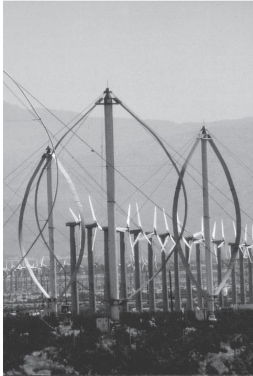
**Figure 1.30** Fixed-speed 300 kW Darrieus unit with gearing and a conventional generator
