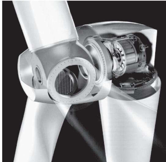
**Figure 1.35** Nacelle of the large-scale Multibrid N 5000 (5 MW, 116 m rotor diameter) with single-stage gearing, integral hub and low-speed synchronous generator. Reproduced by permission of Multibrid Entwicklungsgesellschaft GmbH
