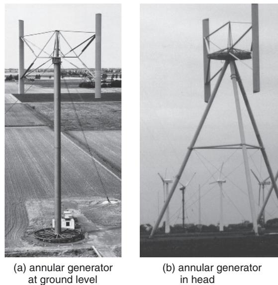
**Figure 1.31** Variable-speed 300 kW gearless H-Darrieus unit
