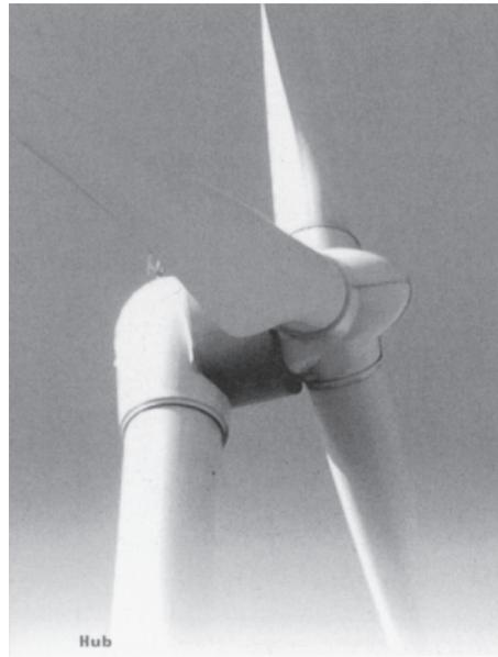
(b) Zephyros Z72 (70.65 m rotor diameter and 2 MW nominal output) with medium-voltage generator. Reproduced by permission of Harakosan
