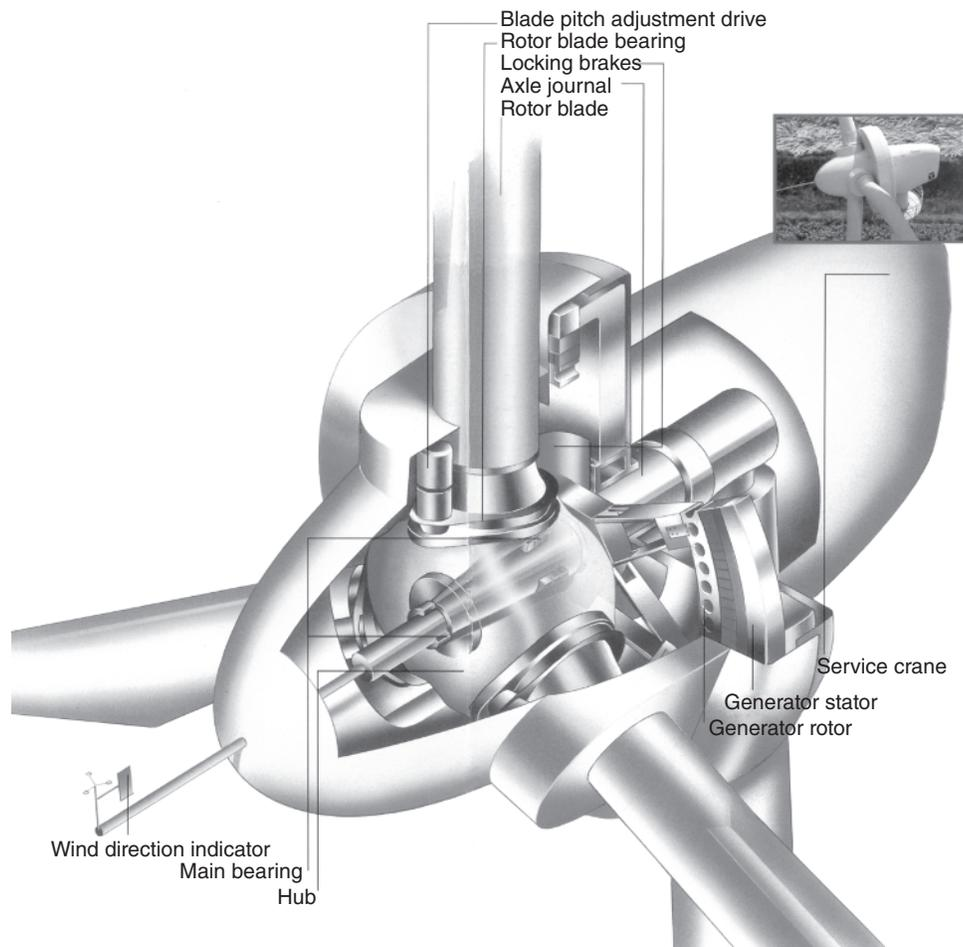
**Figure 1.32** Schematic layout of the Enercon E 40 gearless turbine. Reproduced by kind permission of Enercon
