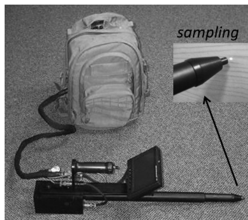
Figure 1.8 A person-portable LIBS unit for analyzing surfaces. The tip of the probe is placed on the surface and the laser is fired to record a spectrum (ca. 2010).
