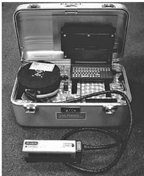
Figure 1.7 A portable LIBS surface analyzer, circa 1995. (Reprinted with permission from Yamamoto et al. (1996).
