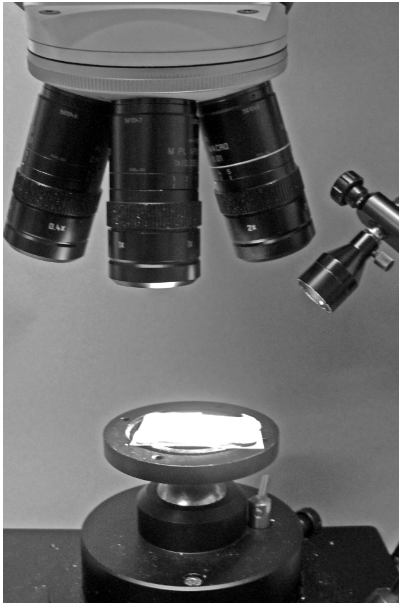
Figure 1.4 A tool mark cast illuminated on a comparator stage. For most tool mark examinations the light will normally be at a shallow angle, rather than at 45° as shown here.
