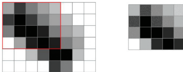
Figure 1.10 Image cropping. An area is selected and the rest of the image is cropped out leaving the remaining portion unchanged.
