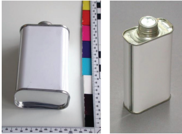
Figure 1.5 Colour scales (and linear scales) provide standard references, against which objects in the image may be compared.
