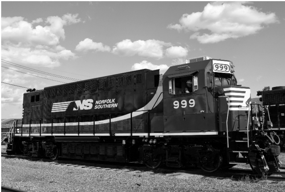
Figure 1.2 Norfolk Southern Electric switchyard locomotive, NS999 (photo courtesy of Norfolk Southern Corp.)
