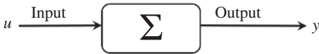
Figure 1.1 A general characterization of a system as an object or process that transforms inputs u to outputs y .
