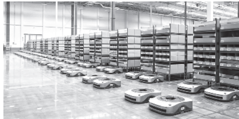
Figure 1.9 Warehouse robots for order retrieval are an example of factory automation, where the robots act with little or no human supervision.
