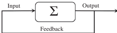
Figure 1.8 A feedback system is one where the output affects future inputs.
