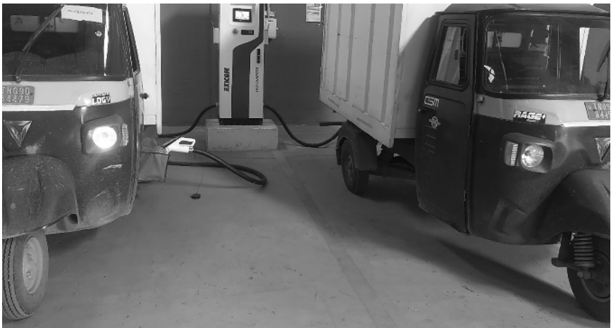
Figure 1.16 DC fast charger 30 kW charging two EVs at a time.
