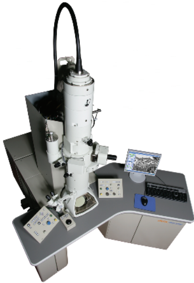
Figure 1.2 Transmission electron microscope. This is a microscope in which the image is formed by electrons transmitted through the specimen.
