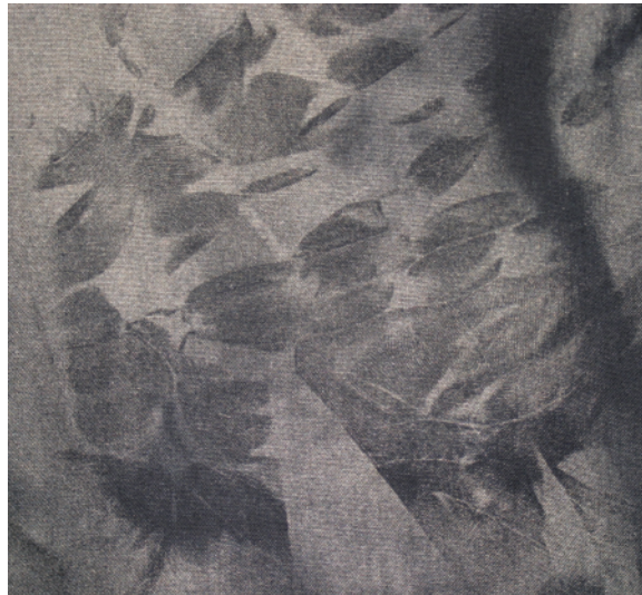
Figure 1.1 A contact (grab) mark on a black cotton shirt developed using vacuum metal deposition. Reproduced courtesy of the Home Office.
