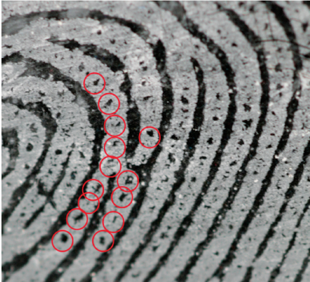
Figure 1.8 A fingerprint enhanced using white powder suspension showing level 3 details (in this case pores, illustrated using circles) in the ridges.
