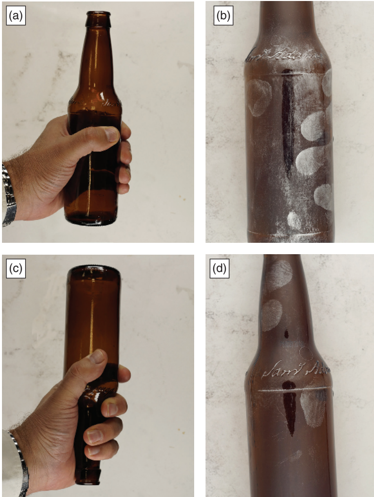
Figure 1.2 The orientation of fingermarks on a glass bottle originating from different actions. (a) Bottle being held to drink from. (b) Fingermarks developed using aluminium powder after drinking. (c) Bottle being held as if to strike. (d) Fingermarks developed using aluminium powder after use as a weapon.
