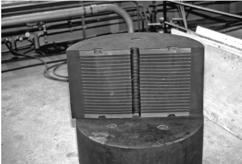
Figure 1.6 Natural rubber isolator for the Foothill Communities Law and Justice Center showing laminated construction. Courtesy of James M. Kelly, NISEE Online Archive, University of California, Berkeley
