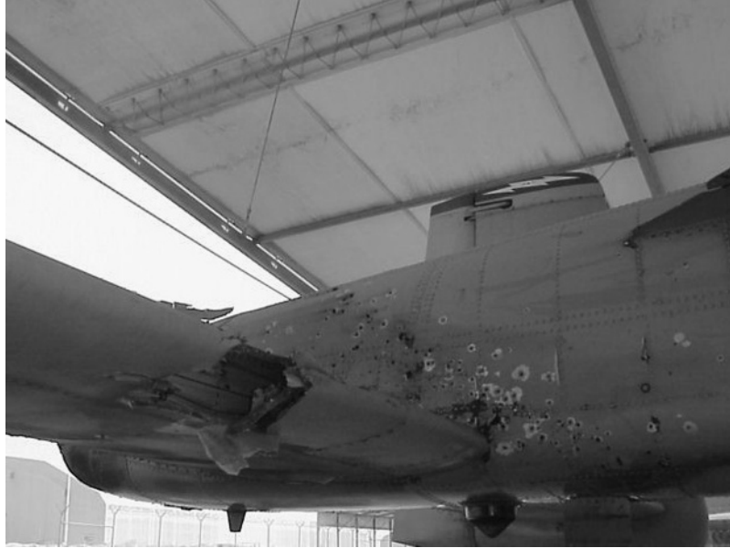
Figure 1.2 Damage sustained by an A-10 Thunderbolt during a 2003 Iraq War mission (source: US Air Force).
