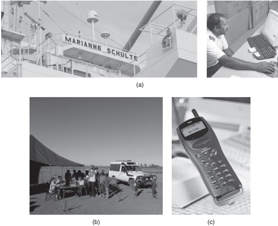
Figure 1.6 (a) A typical large ship-borne earth station configuration – antennas enclosed in radome above deck (left) and an application in progress below deck (right). (b) A typical portable terminal in use in a remote area. (Parts (a) and (b) source: www.Inmarsat.com . Reproduced with permission of Inmarsat.) (c) A tri-mode hand-held terminal supporting satellite, analogue and CDMA digital with 2.5–4.5 h talk time and 9–14 h standby time. (Source: Globalstar. Reproduced with permission of Globalstar.)
