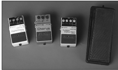
FIGURE 1-3: Four common electronic effects used by guitarists (left to right): digital delay, chorus, distortion, wah-wah.
