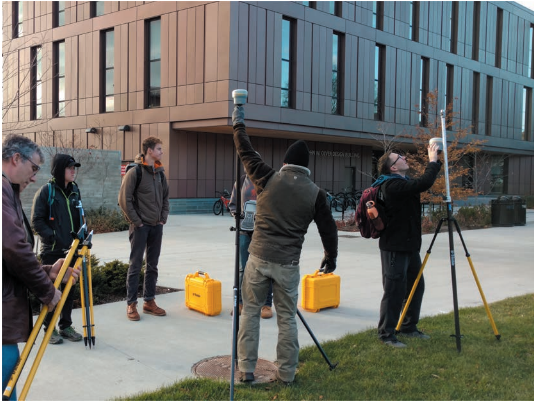
Figure 1.10: Trimble's R10 GNSS units in action during a workshop at the UMass Amherst Trimble Technology Lab
