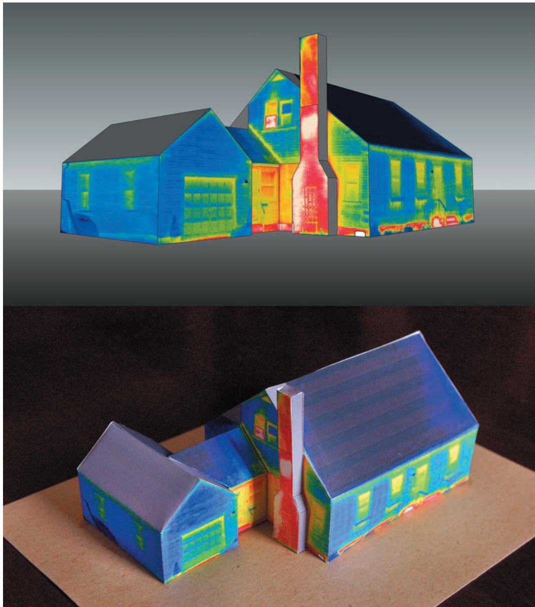
Figure 1.6: Thermal infrared house model made in SketchUp (top) and physically built as a paper model using extensions (bottom). For this project, images from a thermal infrared camera were pasted as textures to all surfaces using SketchUp's texture positioning tools
