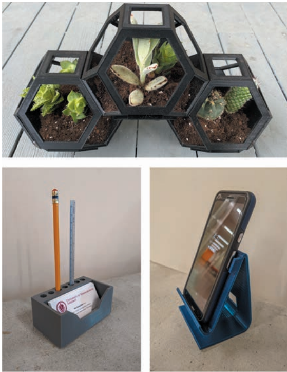
Figure 1.18: Three items designed by my students in SketchUp and then 3D printed
