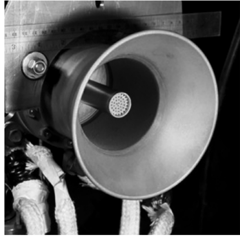
Figure 1-6 Example of a laboratory self-field MPD thruster (Source: Photo credit: E. Choueiri, Princeton University).
