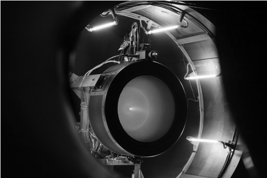
Figure 1-2 Photograph of the NEXT ion thruster during thermo-vac testing at JPL (Source: NASA/JPL, Public Domain).
