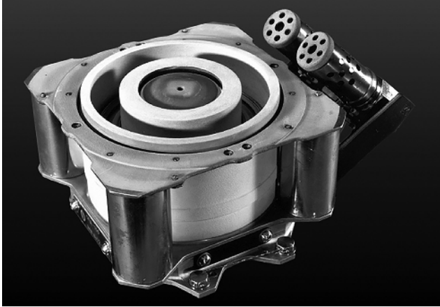
Figure 1-4 Photograph of the SPT-100 Hall thruster ( Source: [27]/American Institute of Aeronautics and Astronautics, Inc. ).
