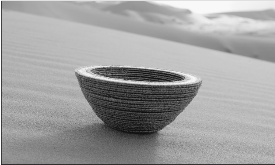
FIGURE 1-3: A glass bowl formed by passing sunlight through the Solar Sinter to fuse sand.
