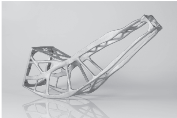
FIGURE 1.14 High-strength aluminum antenna bracket for a space satellite produced by additive manufacturing. The part is approximately 40 cm (16 in.) in length and weighs less than 1 kg (2.2 lbs). (Courtesy of EOS GmbH.)
