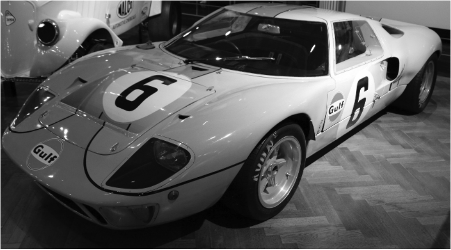
The 1968 Ford GT40. The car was named GT for Grand Touring, with the 40 representing its overall height of 40 inches.
