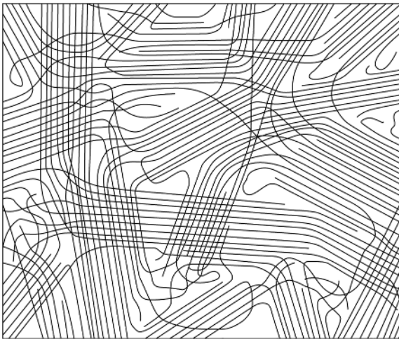
Figure 1.13 The fringed micelle representation of crystalline polymers. Adapted from Hill, 1953.
