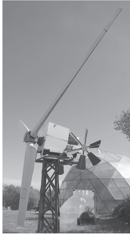
Figure 1.12 Økær 5-m-long fiberglass blades on a 22 kW Smedemestermølle of the Riisager type. Note the blades turn in a clockwise direction. Restored and displayed at the Renewable Energy Museum, Denmark.
