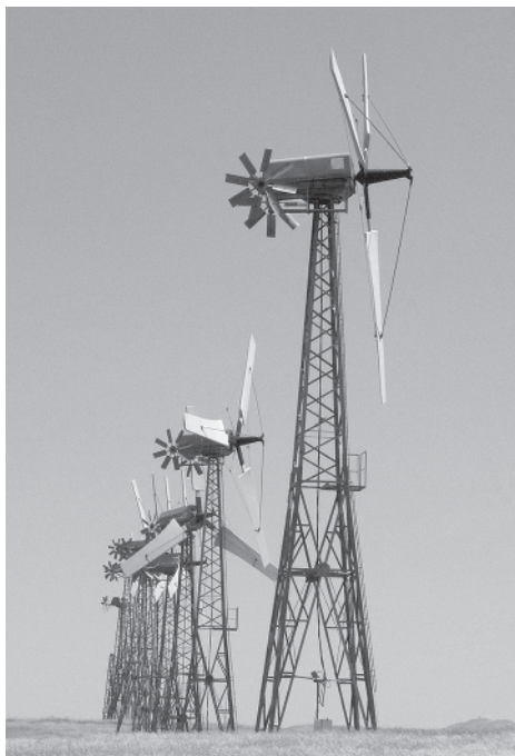
Windmatic 65 kW turbines with 14-m-diameter rotors and hub height of 18 m. Designed by Christian Riisager. In the former Los Vaqueros Windfarm, north of Livermore, California, as they appeared in 2012.
