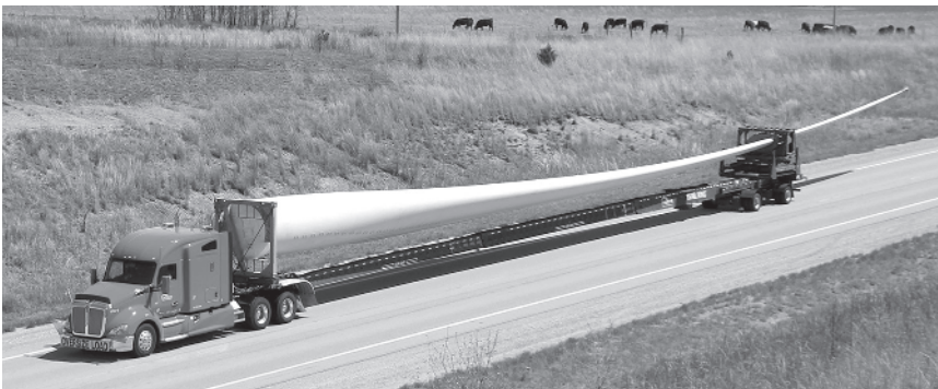
Figure 1.21 Turbine-blade logistics in Kansas. (A) Highway transport by oversized tractor-trailer truck; blades are typically about 50–60 m long, (B) temporary storage in the BNSF Railway depot at Emporia. Vertical view of Gamesa blades in tight-packing arrangement. Service truck shows size of blades. Kite aerial photograph with D. Leiker.
